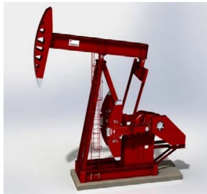
Figure 4. This shows a typical pump jack design with counterweights. ( GRABCAD )
