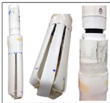
Figure 1. Foot valve filter designed by the previous senior design team.
