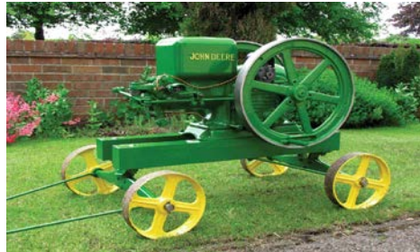
Figure 3. This image shows the use of a flywheel on an antique engine. ( Gas Engine Magazine )
