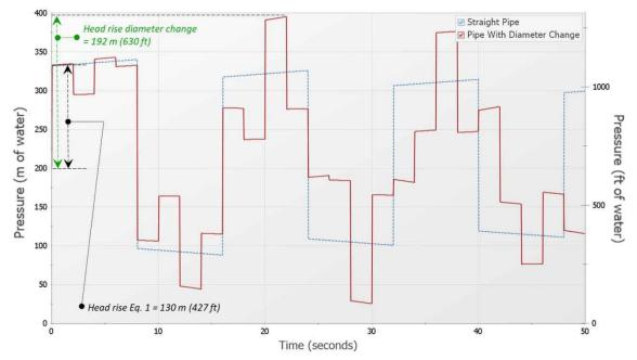
Figure 12: Example 5 - Simulation results for Figs. 7 and 10 at the valve for straight pipe and pipe with diameter change systems.
