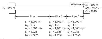
Figure 7: Example 4 – Straight piping system
