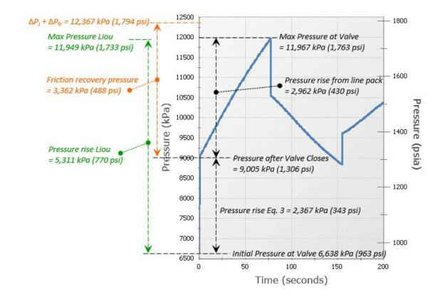
Figure 5: Example 3 – Predicted pressure transient at the valve from the system shown in Fig. 3 for 200 s with additional details on the various pressure rise estimation methods
