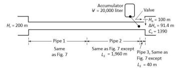
Figure 14: Example 7 - Piping system with a gas accumulator
