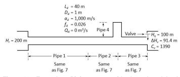
Figure 11: Example 6 - Piping system with a branch and dead end
