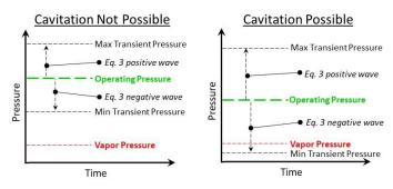
Figure 2: Diagram to help determine the possibility of transient cavitation
