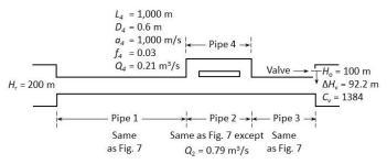
Figure 8: Example 4 - Networked piping system
