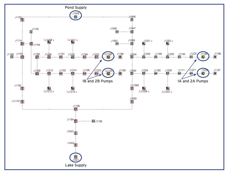
McGuire Nuclear Station RN pump NPSH hydraulic model
